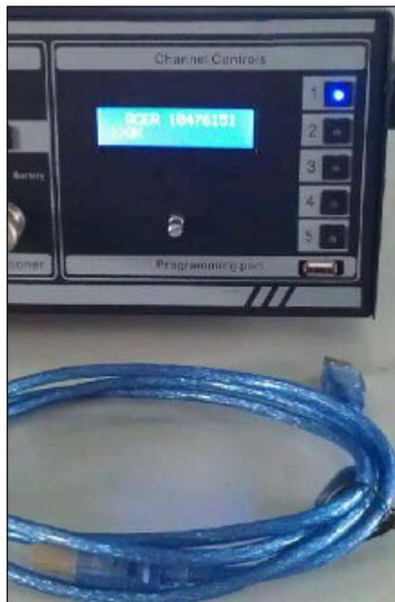
3. Select the correct COM port number in the communications set up area and press the “Connect” push button, the background color of the area should change from Red to Green to indicate communications between the devices is
