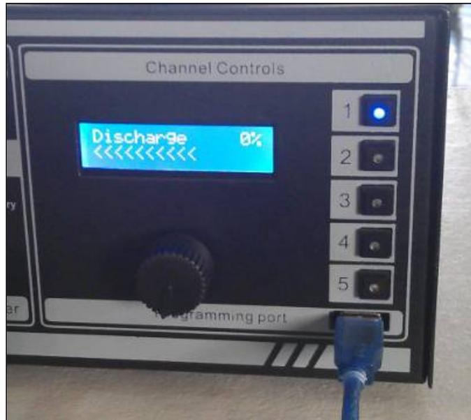
4. Connect the USB cable to PC's USB port
