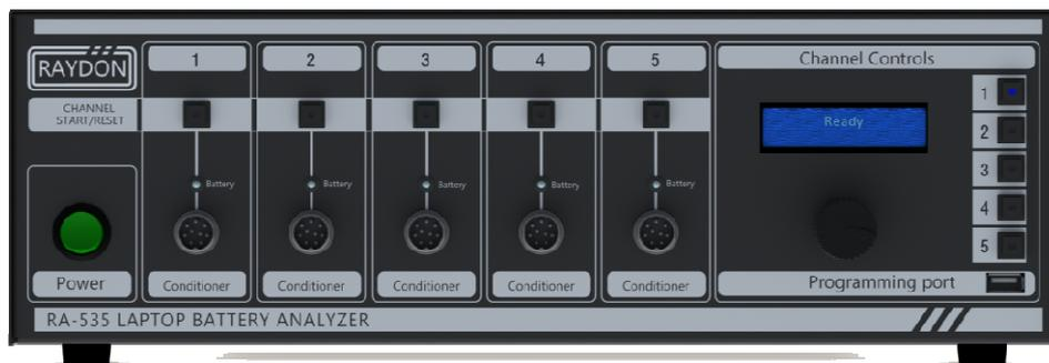
At this time check the all other LEDs on the front panel should be OFF, except Channel Selection Button for Channel #1, which indicates channel 1 is selected as default. BTI-850B should go through an initialization stage, at this stage, the LCD display will show as following:
