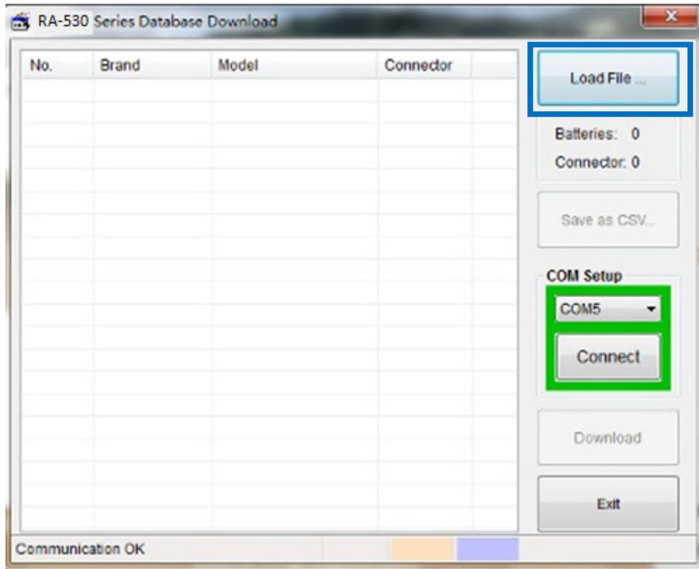
5. A “Select Database” dialogue will appear and user should browses through the storage and locates the location of the database file ready for downloading. Select the file and press “Open” to load the database file.
