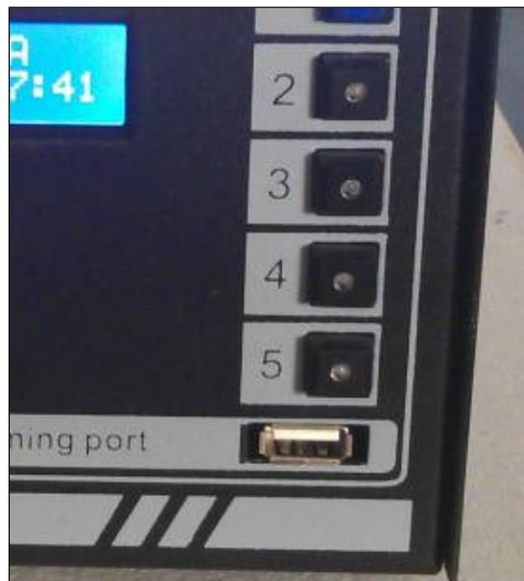
3. Plug the USB cable directly into RA-530 USB Programming Port.
