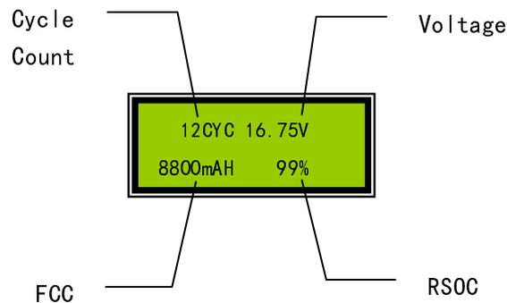
These SMBus Register values will indicate the status of the battery; they are (as defined by SMBus Datasheet):
