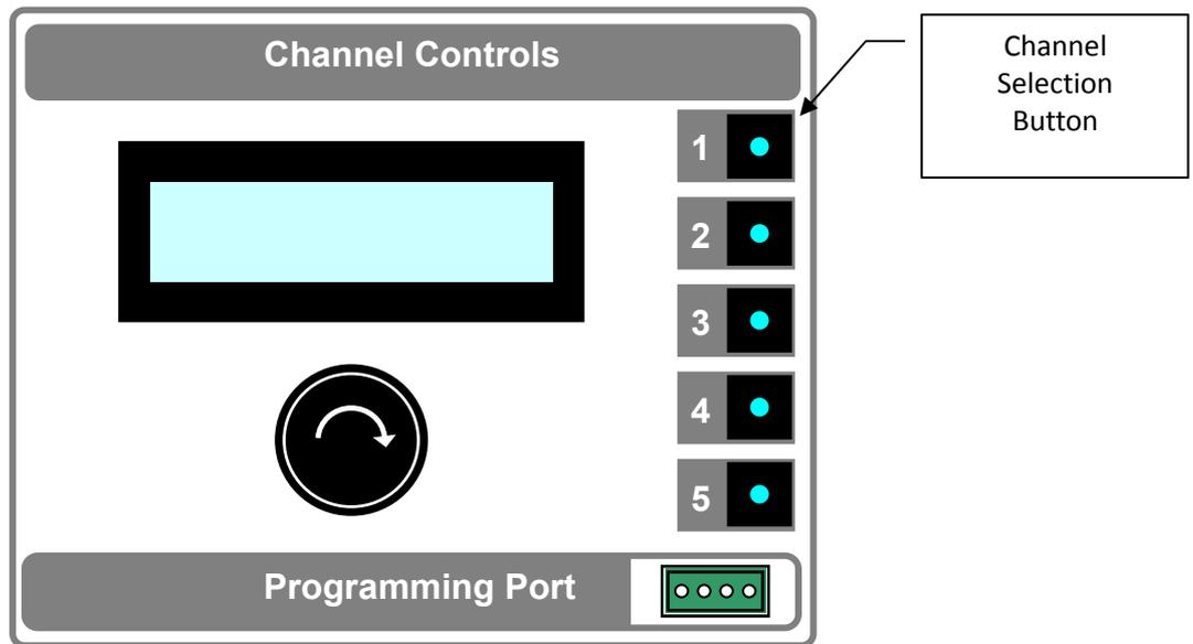
All Channel Selection Buttons have build-in LED to indicate the selected channel. User can use these buttons to switch controls among all 5 channels in the equipment.
